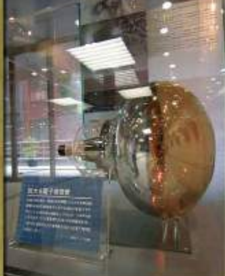
Photomultiplier tube used in the Nobel prize-winning KAMIOKANDE neutrino observatory
