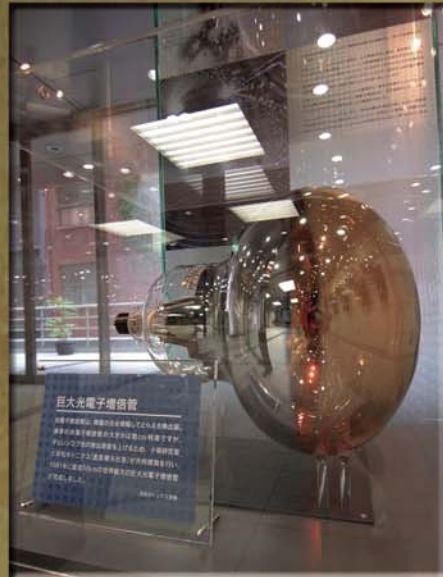
The photomultiplier used in the Nobel Prize winning KAMIOKANDE neutrino observatory.
