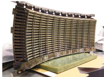
図 6.2.12: 200 MHz combline antenna for TST-2.
