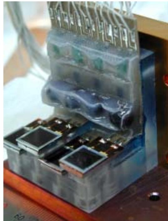
図 2.5 c: PIN photodiodes Hamamatsu S3590-06 assembled with head amplifiers
