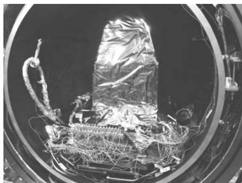
図 6.1.10: Tests at ISAS/JAXA. (top) A vibration test for a BGO block used in the SGD, performed on 2011 September 9. (bottom) A thermal dummy of the HXI detector, about to be tested inside a vacuum chamber.
